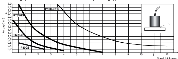
Max. air gap between sensor and first sheet (1st air gap)
